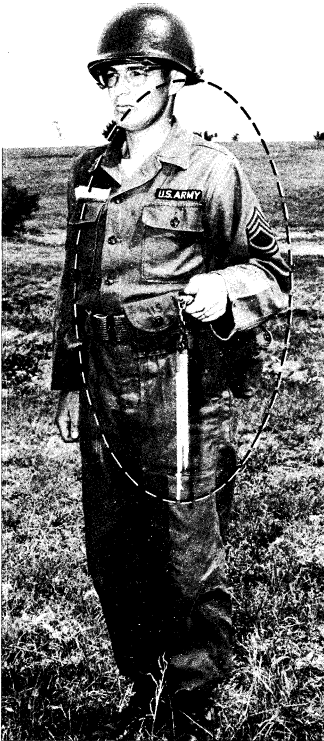
Figure 32. Ventilation of psychrometer.
