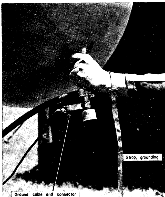
Figure 35. Grounding of hydrogen generating equipment.
